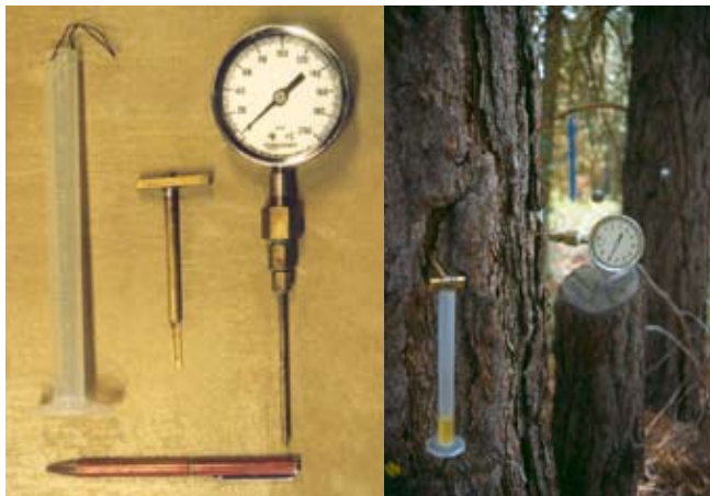
Resin flow and pressure equipment used in this study. (A) From bottom to top: 25 mL cylinder, brass “scoop,” and pressure gauge (with nipple attached). The pen is shown for scale. (B) Oleoresin exudation pressure (OEP) and oleoresin flow (OEF) measurements in a pole-size ponderosa pine. (Permission from Canadian Journal of Forest Research, 2006.)
